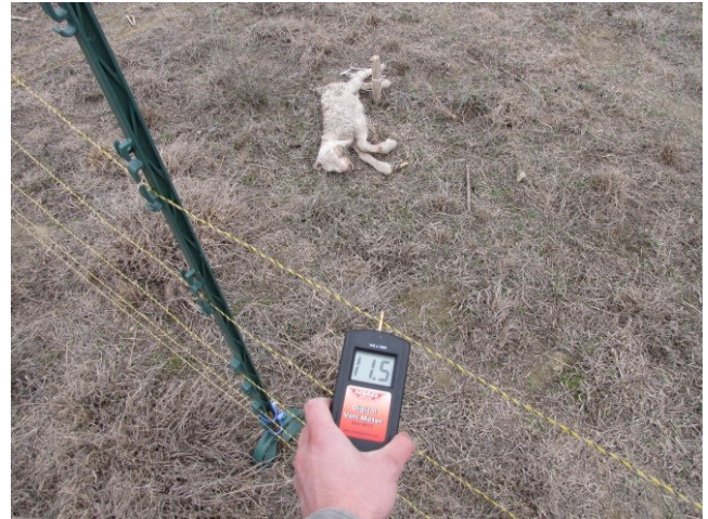
Figure36: Measuring voltage in wires at experimental fence with bait and camera traps
